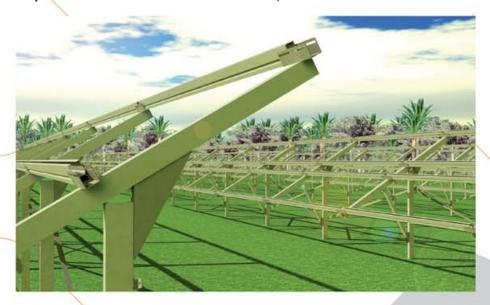
The fixing of the panels to the metallic shapes and the wiring are made in a fast, simple and economic way, because the steel shapes comes with some grooves for the fixing of the screws that can be carried out all along the shape.
