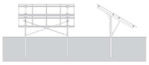
100 % robust, the monopost structure is also able to absorb the unevenness of the ground. With the multipoint system we can adjust it in areas with inclinations of up to 15 %.
